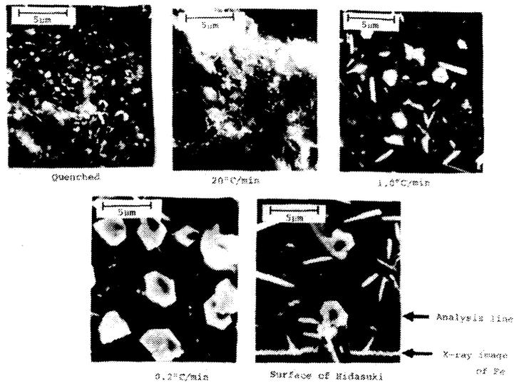
Fig.4 EPMA result and SEM photographs of the surface of samples. Each samples except Hidasuki is a mixture of Bizen-clay and 8wt% KCl.
