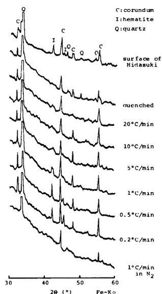
Fig.1 X-ray diffraction patterns of the surface of Hidasuki and Bizen-clay 8wt% KCl added cooled down at various rates after heated at 1300° for 3 hr. (C:corundum,Q:quartz,I:hematite)
