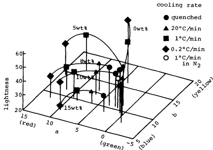
Fig.3 Effect of the amount of KCl added and cooling rate on the coloration of heated Bizen-clay.
