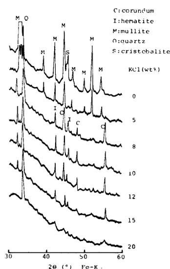
Fig.2 X-ray diffraction patterns of Bizen-clay containing various amount of KCl. All samples were heated at  $1300^{\circ}\text{C}$  for 3 hr and cooled down at  $0.2^{\circ}\text{C}/\text{min}$ . (M:mullite,Q:quartz,S:  $\alpha$ -cristobalite,C:corundum I:hematite)
