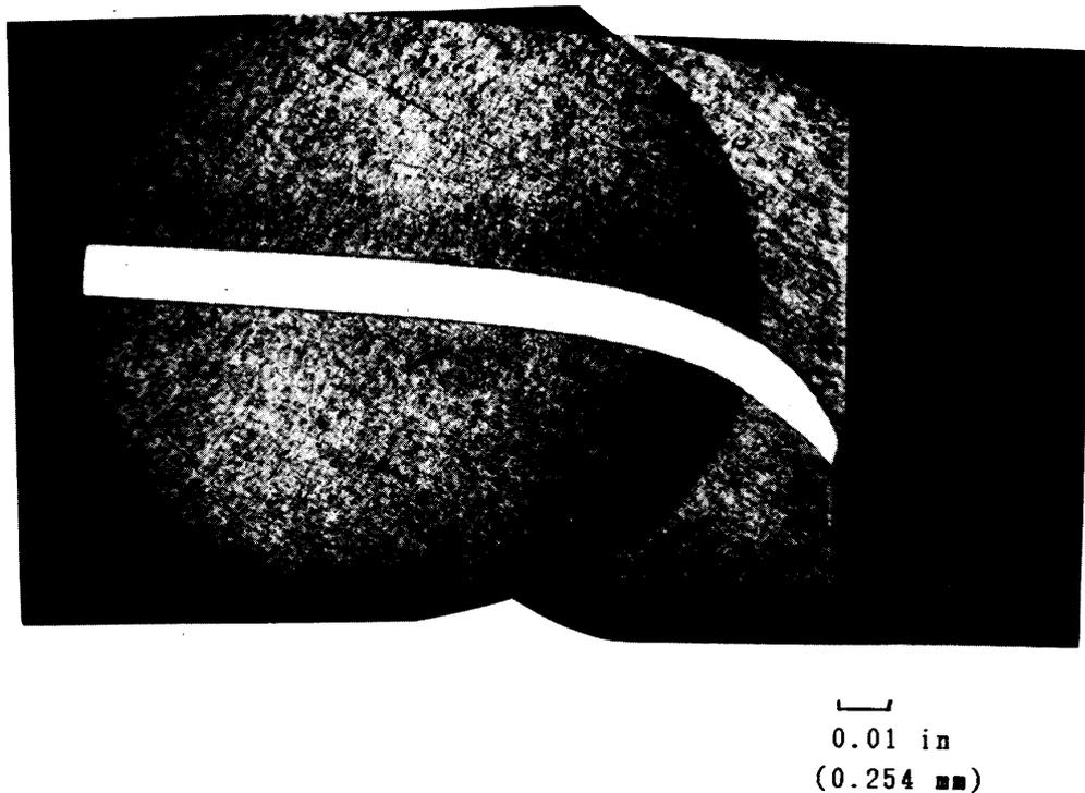
Fig. 5.7 SS-clad Al Sheet Section
