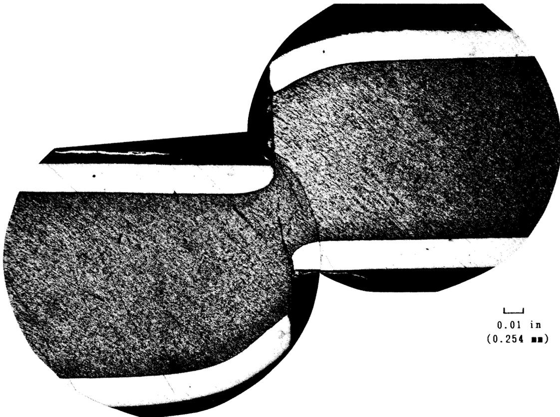
Fig. 5.21 SS-clad Al Half-Way Specimen Section
