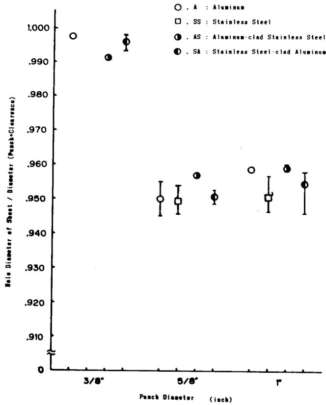
Fig. 5. 2 Ratio of Sheet Diameter to Punch Diameter
