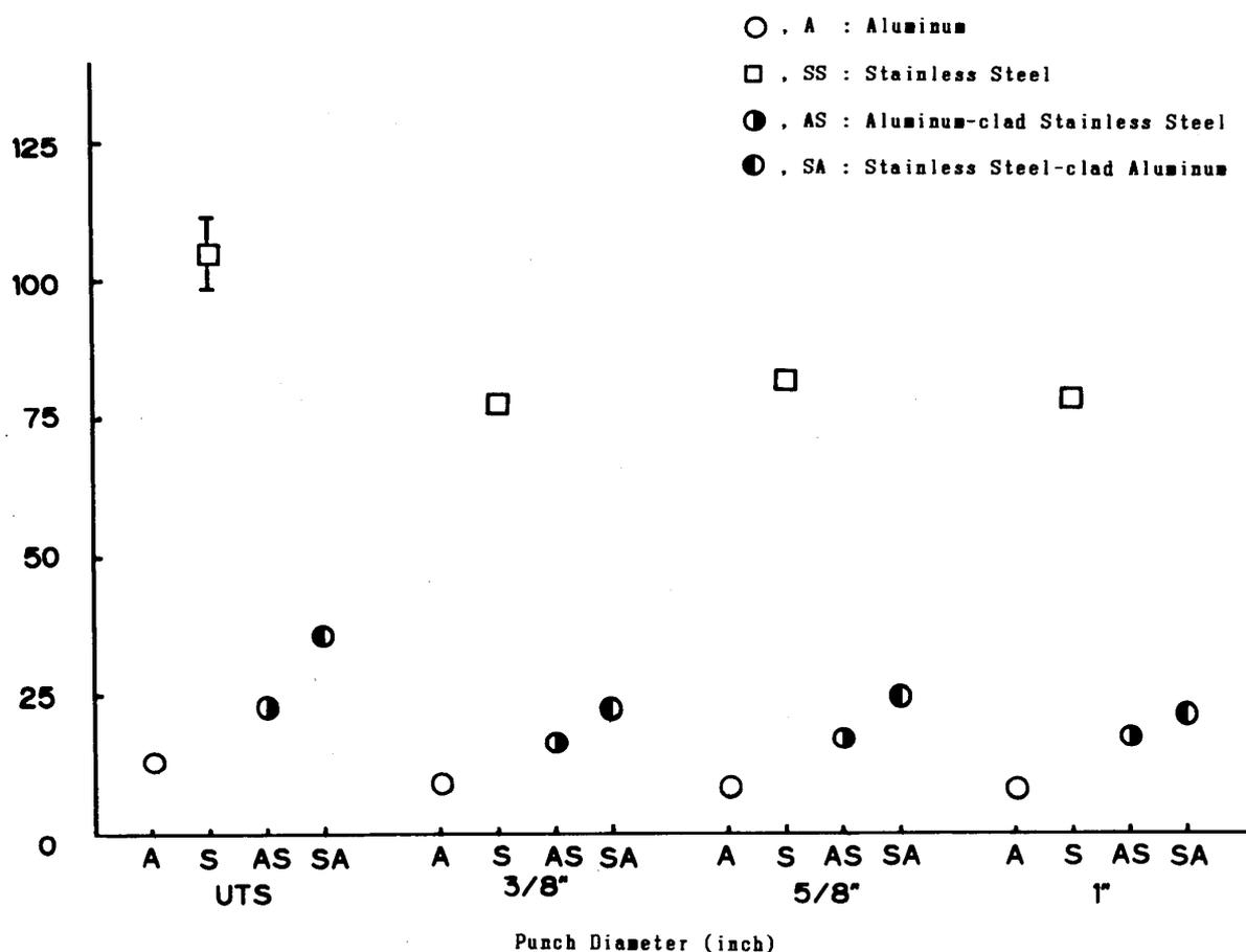
Fig. 5.1 Ultimate Tensile Strength and Maximum Shearing Stress of Each Material in Each Punch Diameter
