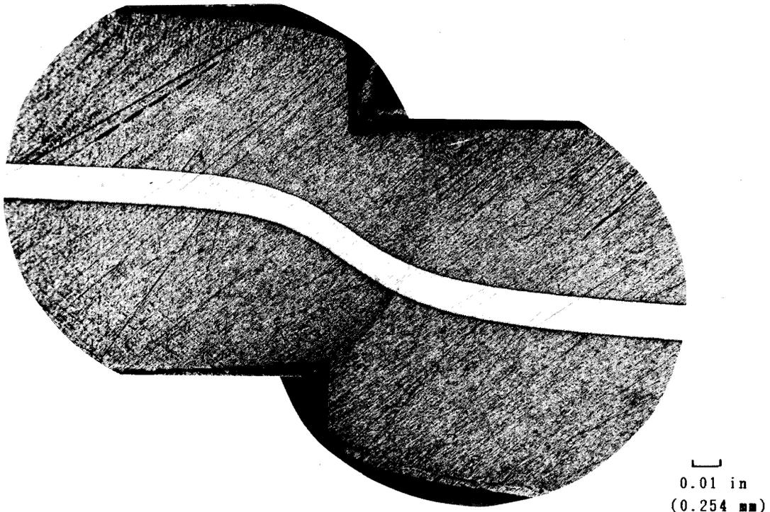
Fig. 5.15 Al-clad SS Half-Way Specimen Section
