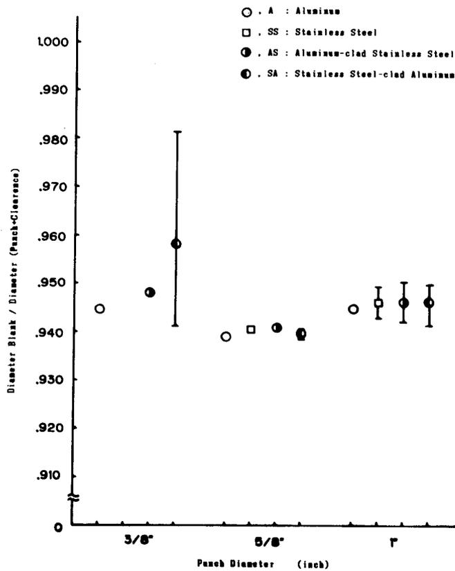
Fig. 5. 3 Ratio of Blank Diameter to Punch Diameter
