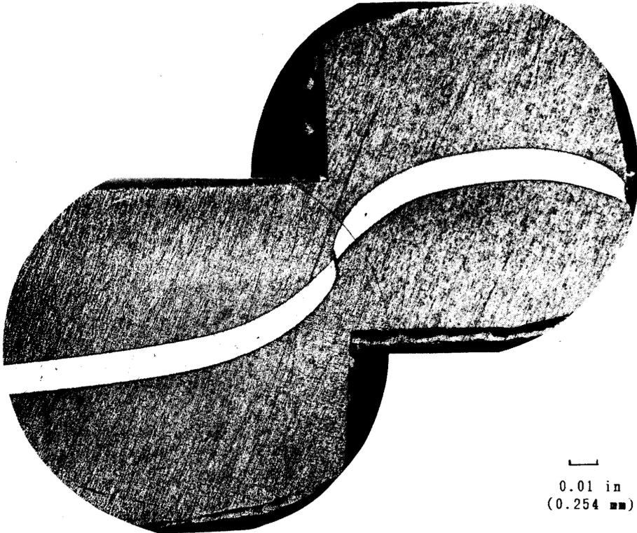
Fig. 5.17 Al-clad SS Half-Way Specimen Section
