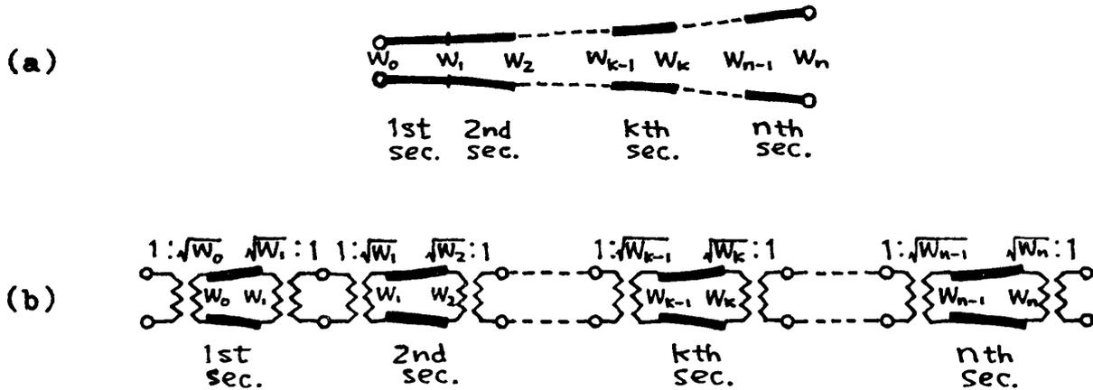
Fig. 2 (a) A section N composed of the cascade of  $n$  self-adjoint transmission line sections. (b) A section equivalent to the normalized section  $\bar{N}$ .
