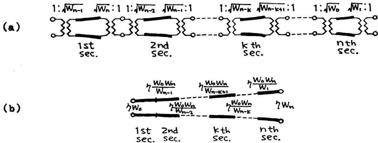
Fig. 3 (a) A section equivalent to the adjoint of the overall section in Fig. 2b. (b) A section equivalent to the adjoint of the section N in Fig. 2a.
