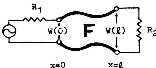
Fig. 4 An impedance-matching system, in which a tapered transmission line is used as a matching section.
