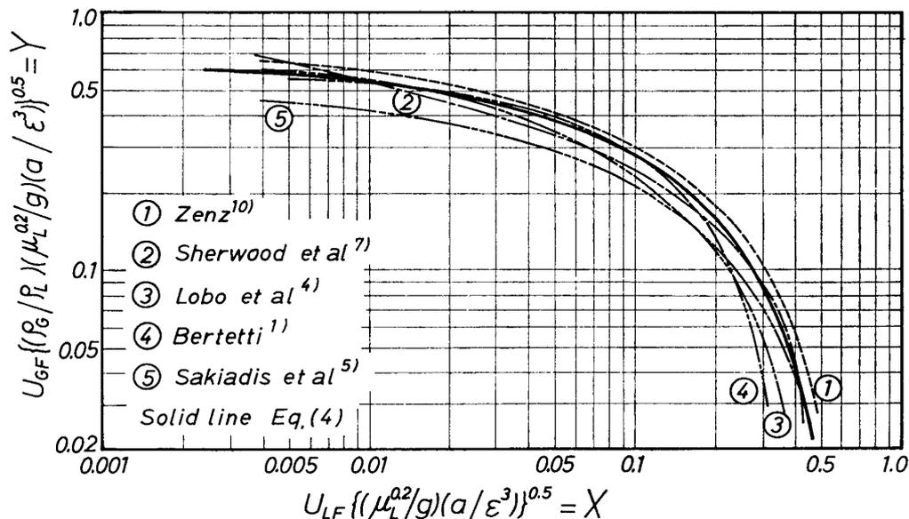
Fig. 1 Correlation of flooding velocities in packed columns
