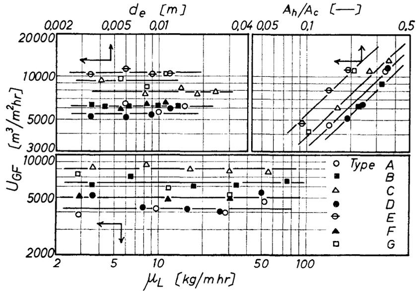
Fig. 5 Effects of  $d_e$ ,  $A_h/A_c$  and  $\mu_L$  for flooding velocities
