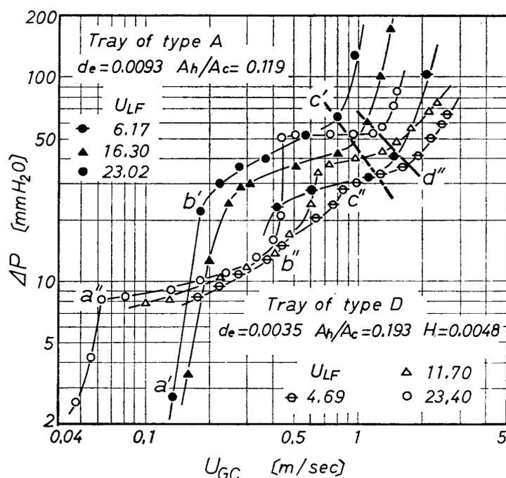
Fig. 4 Typical pressure drop curves in air-water system
