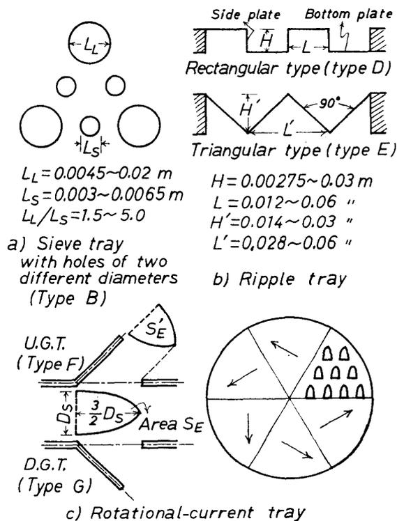
Fig. 2 Structure of trays used
