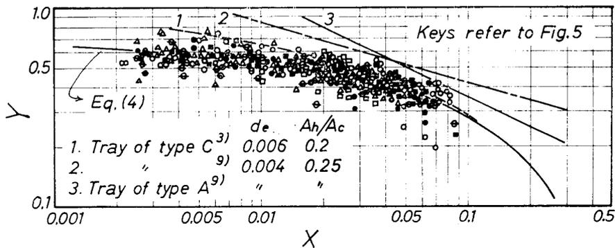
Fig. 7 Comparisons of measured, calculated values and the results of previous works in flooding velocities
