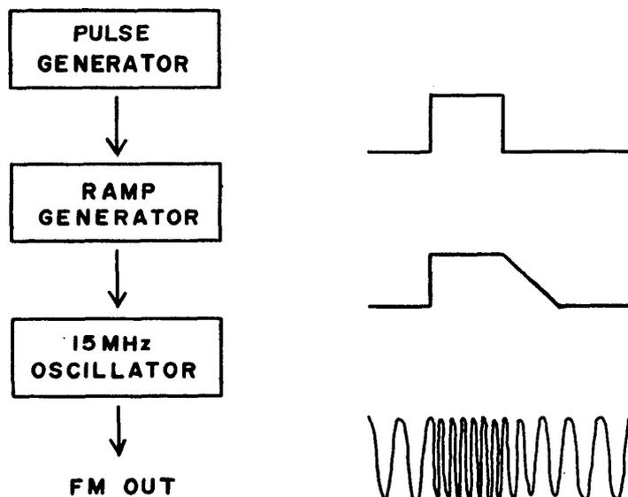
Fig. 1 The block diagram for producing FM wave.
