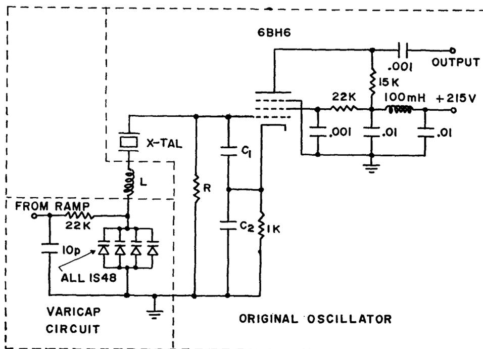
Fig. 2 Schematic diagrams of basic FO-11 international crystal oscillator with modification and varicap circuit. The capacitors marked  $C_1$ ,  $C_2$  and resistor marked R are replaced from original values to 20 pF, 40 pF and 33 K $\Omega$ , respectively and the inductor is added in series with crystal.
