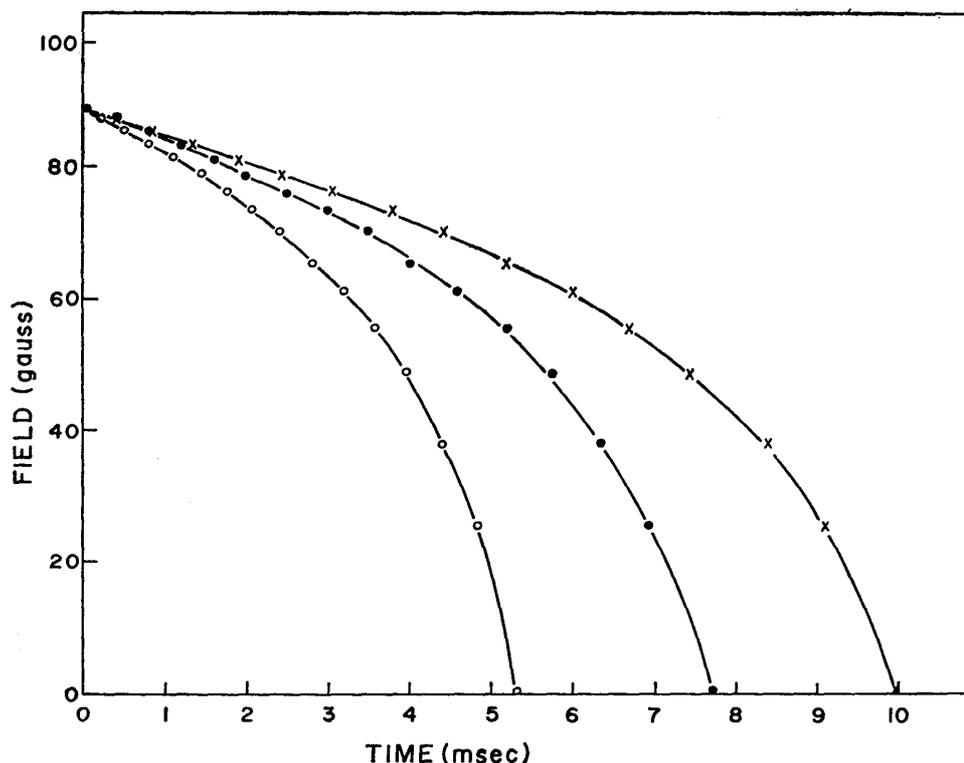
Fig. 3 The field deviation for  $\text{Li}^7$  nucleus plotted against the time following the beginning of the downward ramp. The circles, dots and crosses show the time intervals 5.3, 7.7 and 10.0 msec. during the downward ramp, respectively.
