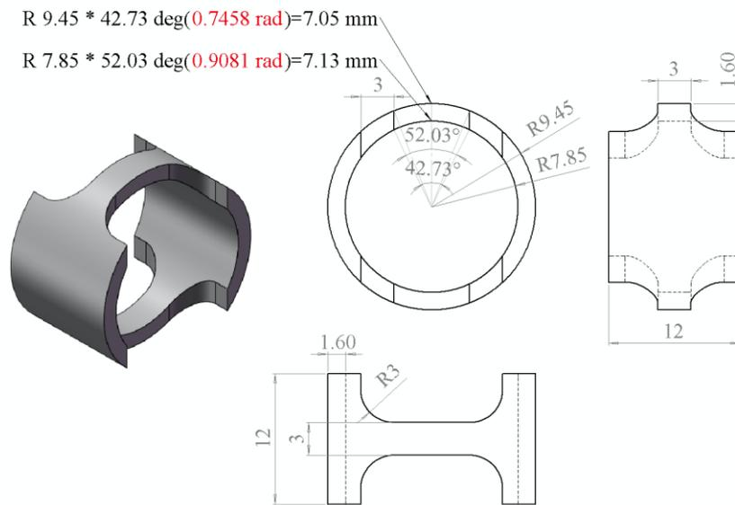
Fig. 4-4 Geometry of specimen for hoop direction tensile test.
