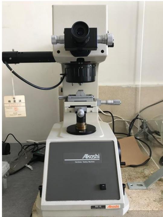
Fig. 3-16 Vickers Hardness tester (Akashi MVK-H0).
