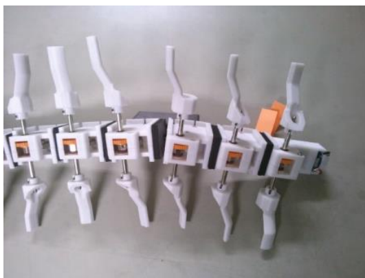
Fig. 2.13 Open space in the ventral side of the body segment
