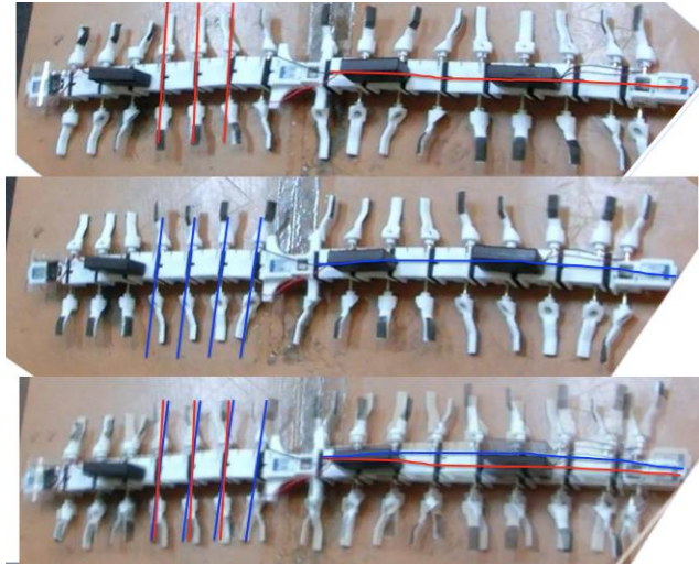
Fig. 2.9 Body undulation of i-CentiPot P
