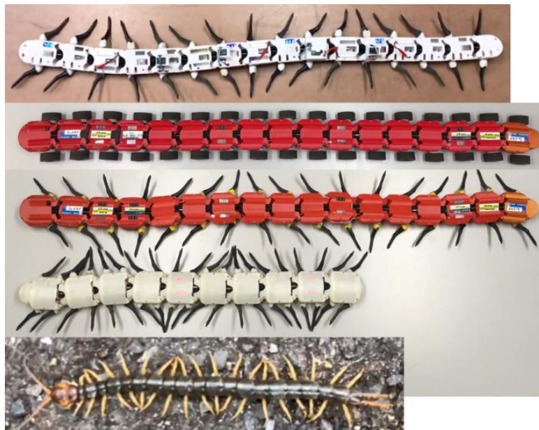
Fig. 8.3 i-CentiPot 01(top), i-CentiPot 02 W(2nd), i-CentiPot 02(3rd), i-CentiPot 03(4th), Scolopendra subspinipes mutilans (bottom)
