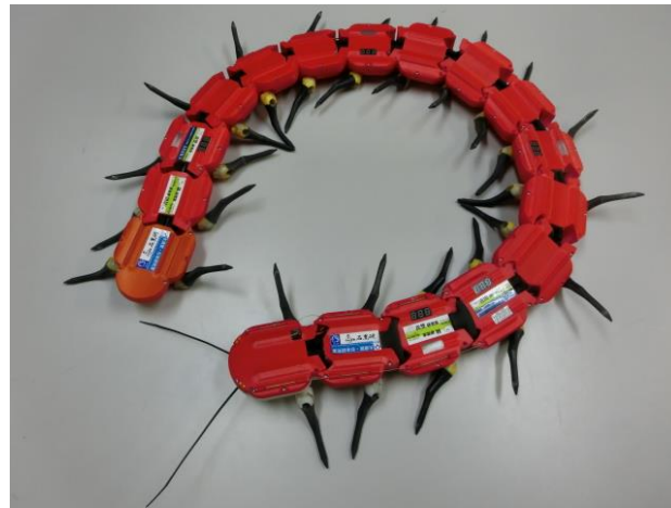
Fig. 5.2 i-CentiPot 02 equipped with an antenna mechanism
