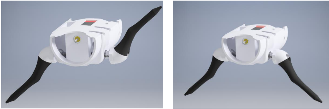
Fig. 3.5 Anti-phase (left) and in-phase (right) of the left and right legs
