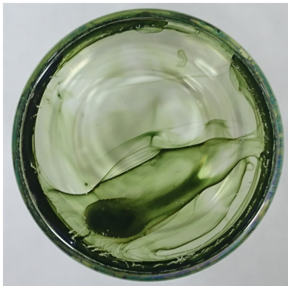
Figure 3-7. A green solid obtained by evaporation of THF solvent
