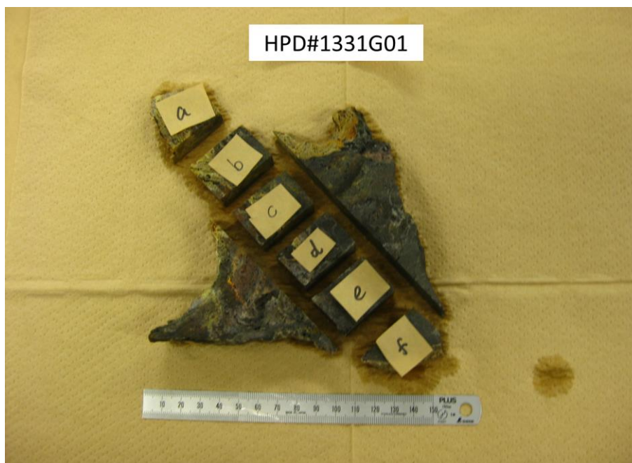
図 3.3 チムニー鉍石を層ごとに切断 (HPD#1331G01)
