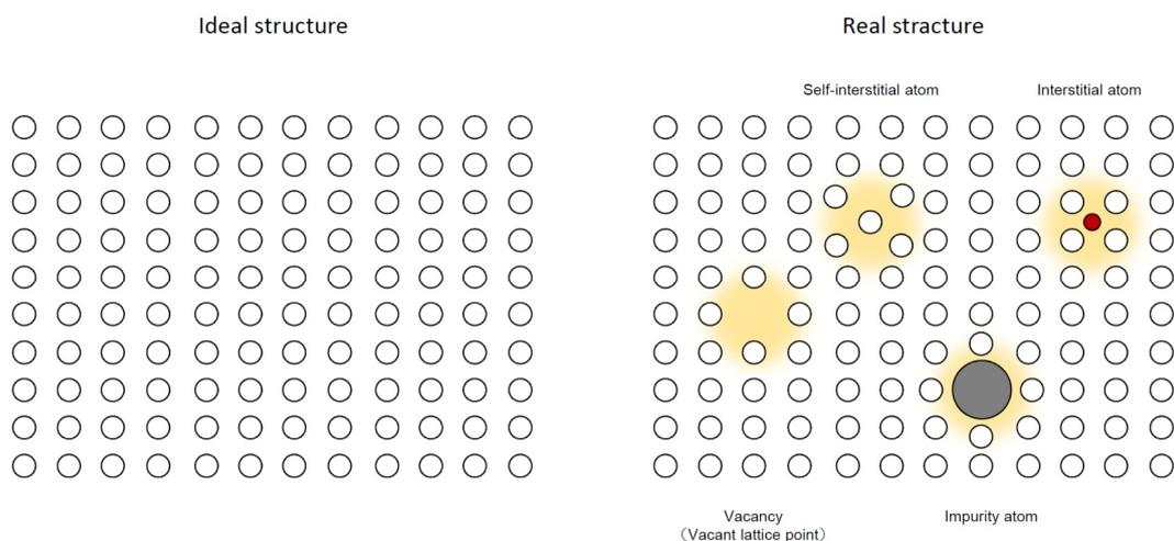
Figure. 1-3 Schematic view point defects of various types, (left) ideal crystal structure, (right) (e.g., vacancy, self-interstitial atom, substitutional impurity atom, interstitial impurity atom).
