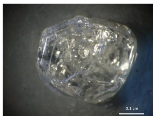
Figure. 3-2 Synthetic zircon formed by flux-fusion method courtesy of Kayama, Kobe University.
