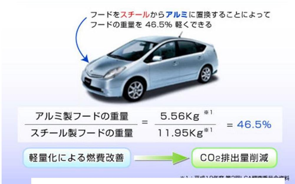
Fig.1-2 The CO<sub>2</sub> emission reduction effect of aluminium application.
