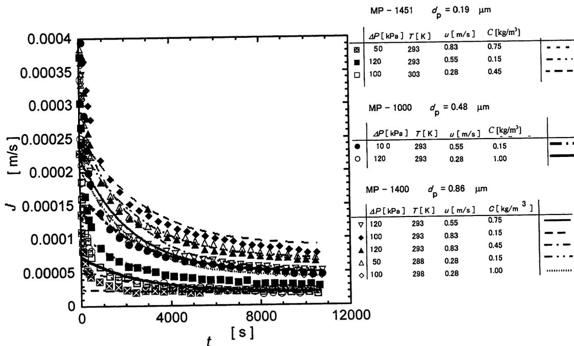
Fig. 6 Comparison of experimental flux decline data with calculated ones
