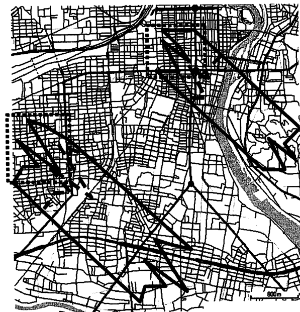
Fig. 7 Regions including the upwind edge to the downwind edge of the source area for each site under (a) stable and (b) unstable conditions in the commercial ( z_0 = 1.0 m) and residential ( z_0 = 0.2 m) spaces. The solid lines represent the areas connecting the edges of source-area length for z/L = 0.1 in (a) and -z/L = 4.0 \times 10^{-4} in (b). The dashed lines represent those connecting upward edges of source area for z/L = 2.0 \times 10^{-4} in (a) and -z/L = 1 in (b).
