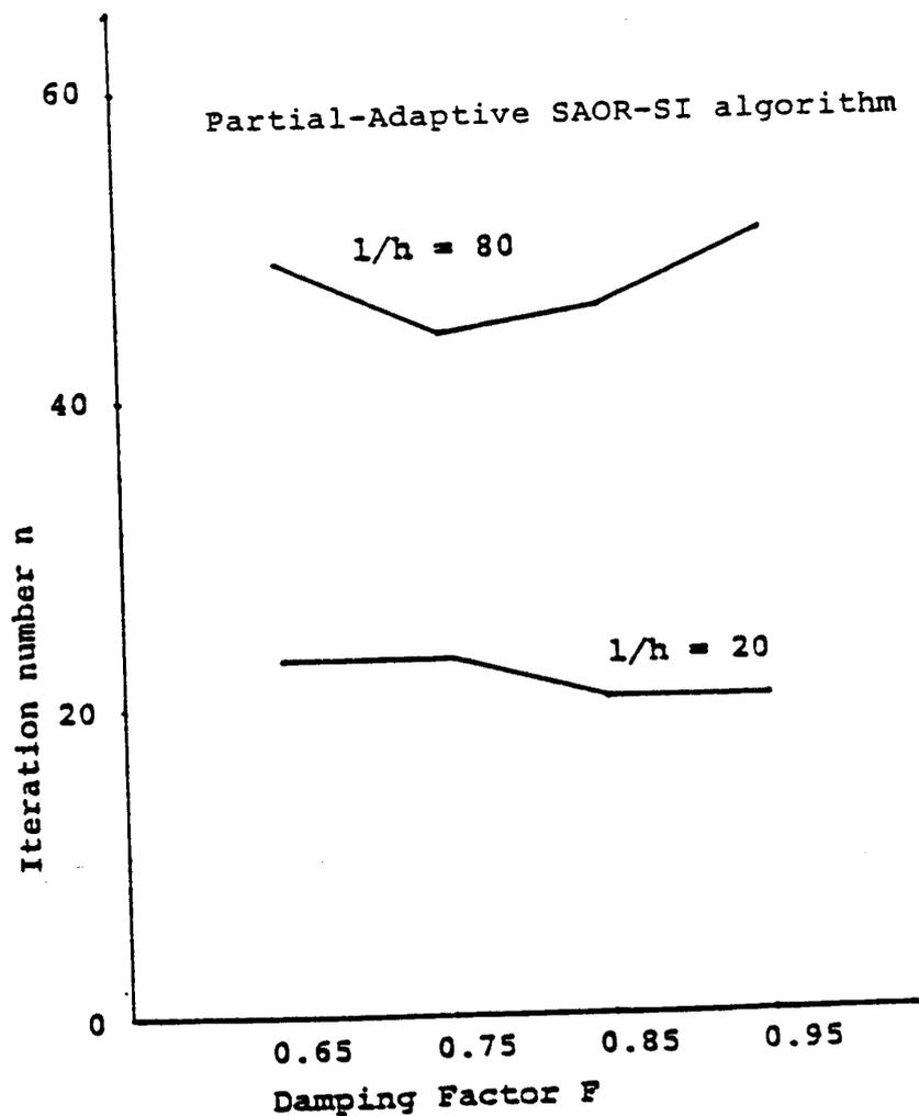
Figure 3: Iteration number versus damping factor for the Partial-Adaptive SAOR-SI algorithm.
