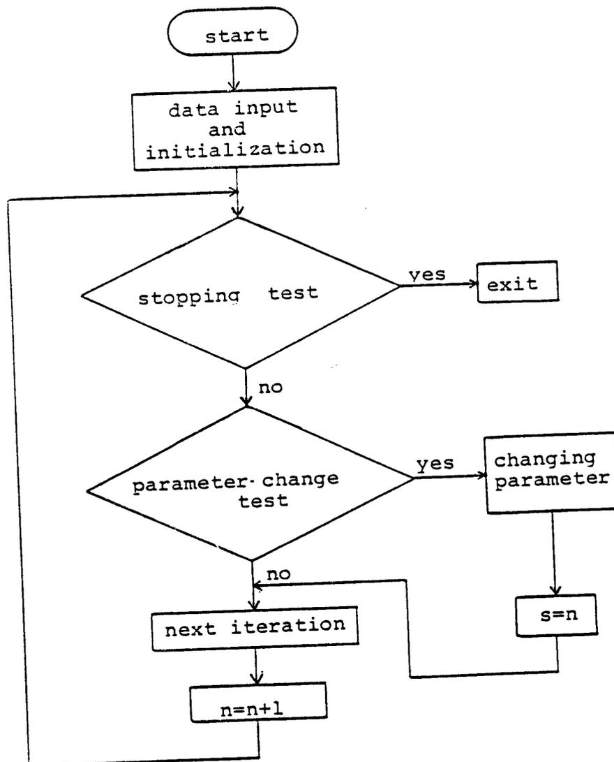
Figure 2: Flowchart of the Partial-Adaptive SAOR-SI algorithm.
