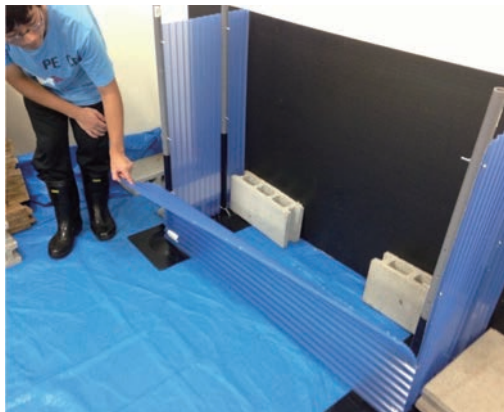
Fig. 3. Warping fence attached to the experimental apparatus. When nutrias hang on the fence, the top of the fence bends.
