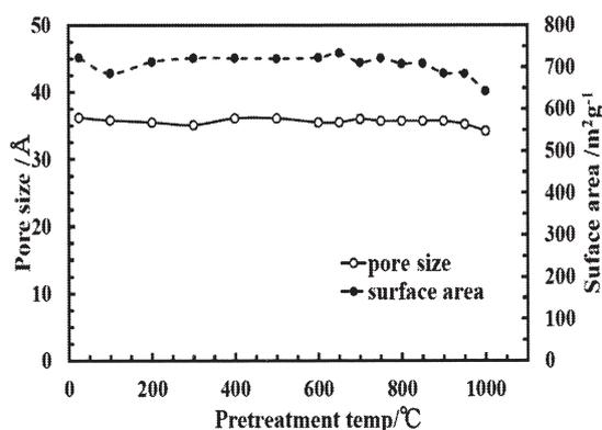
Fig. 1. Effect of heat treatment on the pore size and specific surface area of MCM-41(C18).
