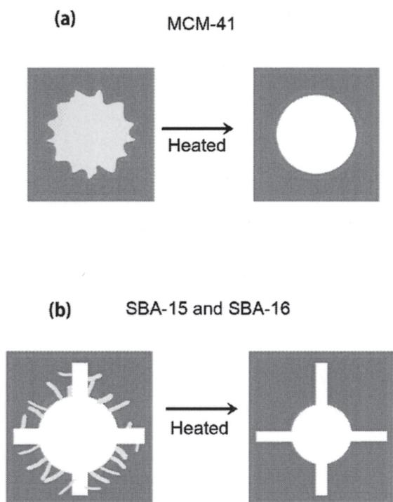
Fig. 6. Images of pore contraction of porous silica by heat treatment. (a) MCM-41(C18), (b) SBA-15 and SBA-16.
