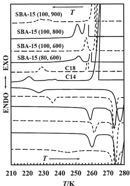
Fig. 3. Low temperature DSC curves of water contacted with MCM-41, SBA-15 (80) and heated SBA-15 (100). Scanning speed is  $5 \text{ Kmin}^{-1}$ . The numbers after the temperature of hydrothermal treatment during preparation are the calcination temperatures ( $^{\circ}\text{C}$ ).
