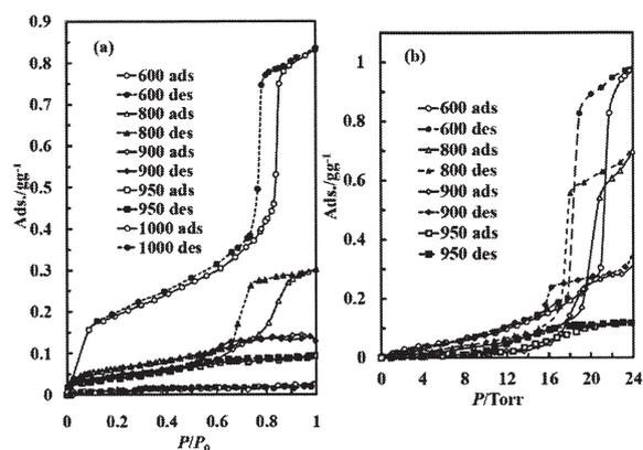
Fig. 2. (a) Adsorption isotherms of nitrogen at the temperature of liquid nitrogen on SBA-15 (120). (b) Adsorption isotherms of water on SBA-15 (120) at 298.2 K.
