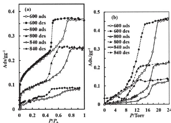
Fig. 4. (a) Adsorption isotherms of nitrogen on SBA-16 (110). (b) Adsorption isotherms of water on SBA-16 (110) at  $298.2 \text{ K}$ .
