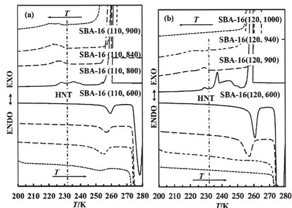
Fig. 5. (a) Low temperature DSC curves of water contacted with SBA-16 (110) heated at increasing temperatures. (b) SBA-16 (120). Scanning speed is  $5 \text{ Kmin}^{-1}$ . The numbers after the temperature of hydrothermal treatment during preparation are the calcination temperatures ( $^{\circ}\text{C}$ ).
